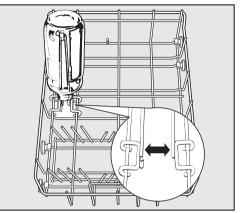
Place the bottle holder in the lower basket as shown. If placed elsewhere, water from the spray jets will not reach the inside of the bottle. The bottles will not be properly cleaned.
